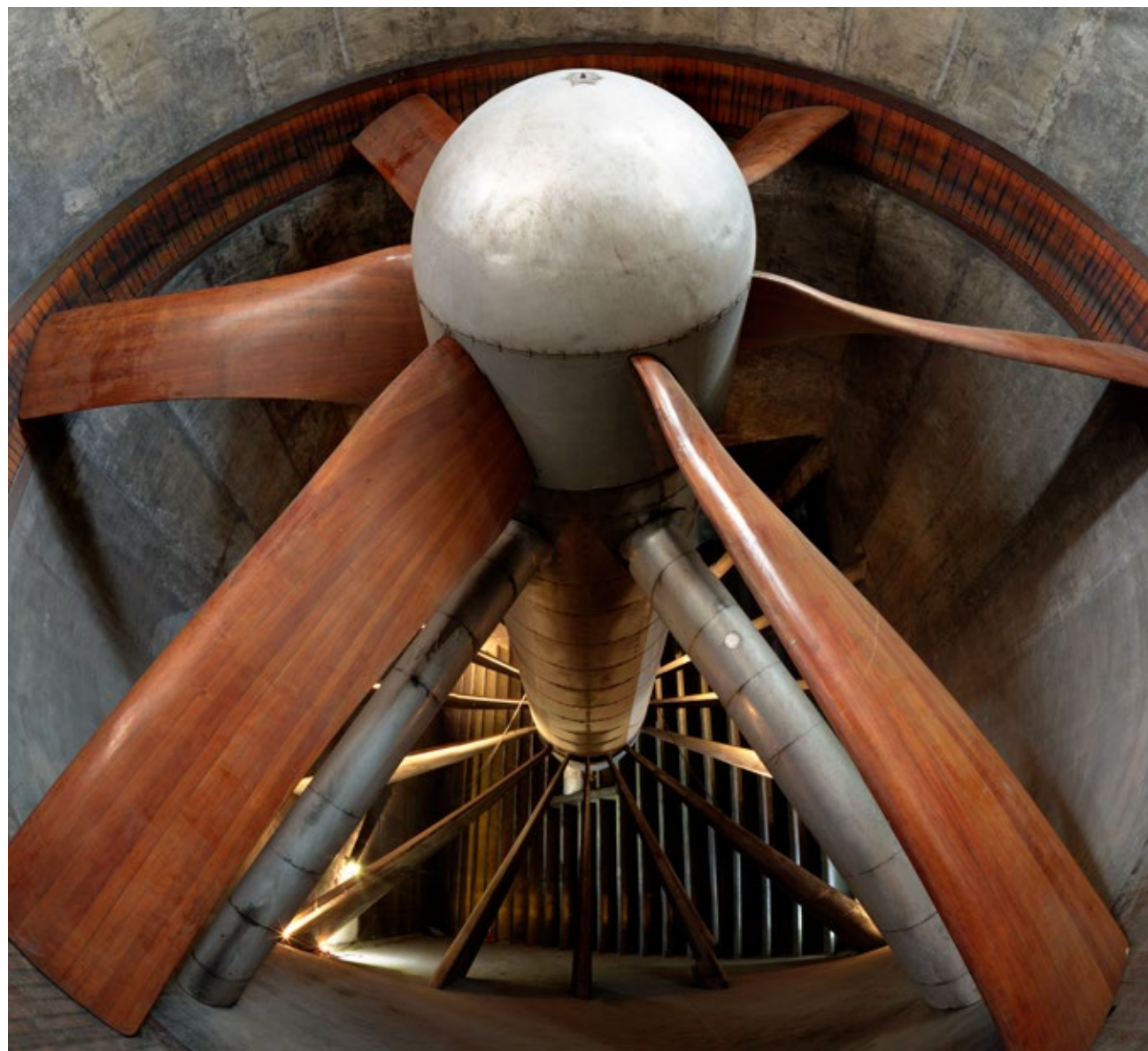
Q121 Fan. The 30' diameter mahogany fan at the start of the Q121 wind tunnel loop, located in Farnborough. Pentax K3 with DA 12-24mm f4 lens. © Matt Emmett
